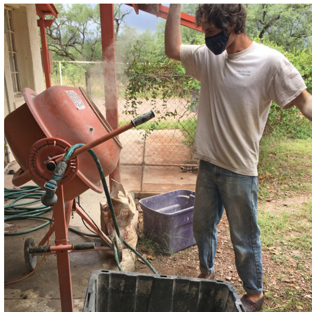
BRN staff uses a small cement mixer to make large batches of seed pellets. The rotating motion naturally encourages the mixture to form spherical structures when the right ratio of dry materials to water is combined.
